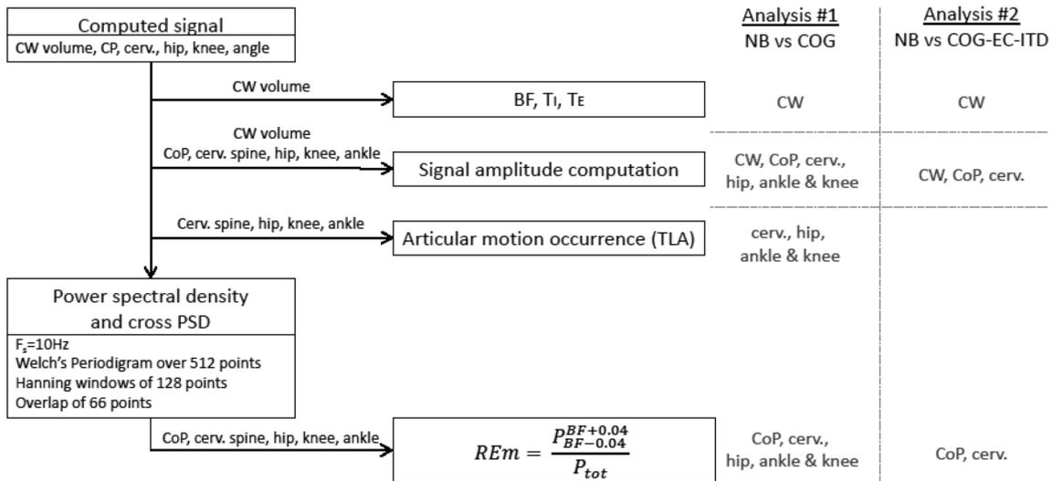
**Fig. 4** Flowchart presenting the computation of each studied variable and its use in analyses 1 and 2. (CW volume chest wall volume, CoP centre of pressure, cerv. spine cervical spine, PSD power spec-
