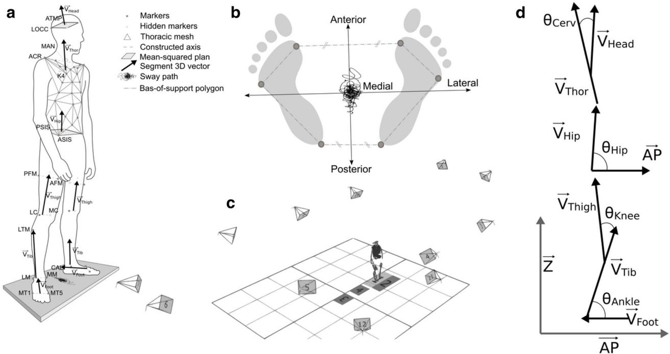
**Fig. 1** **a** Locations of the retroreflective markers and thoracic mesh used to define the body segment frame; **b** definitions of a specific subject's antero-posterior and medio-lateral axes according to the foot markers; **c** positions of the cameras located around the subject; **d** segment vector projected in the sagittal plane and the definition of the articular joint angle ( $\theta$  angle computed for each joint; AP antero-posterior axis, Z vertical axis)
